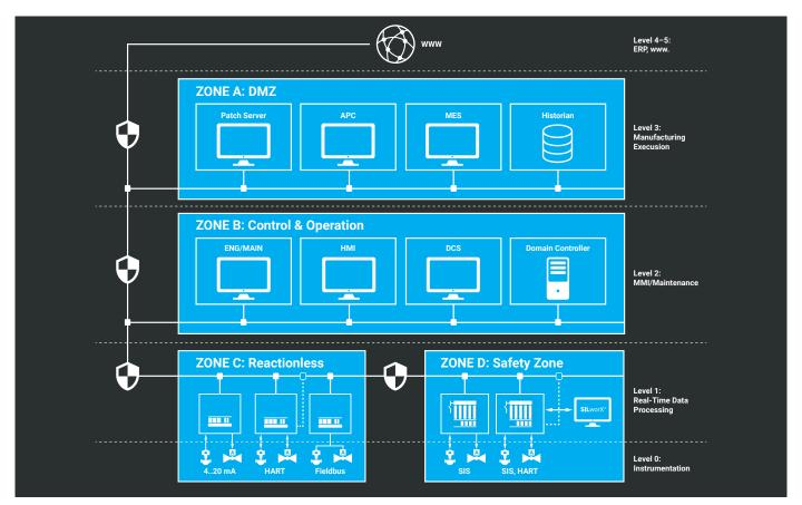
Possible design of zones and conduits for compliance with the IEC 62443 standard
