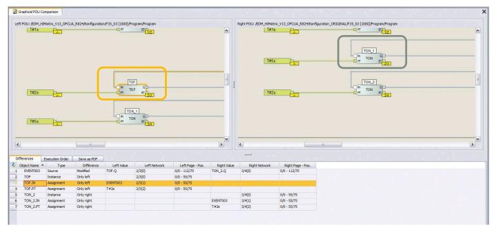
By selecting two different versions of a logic, the differences are highlighted graphically in side-by-side windows and supplemented by details in tabular form.
