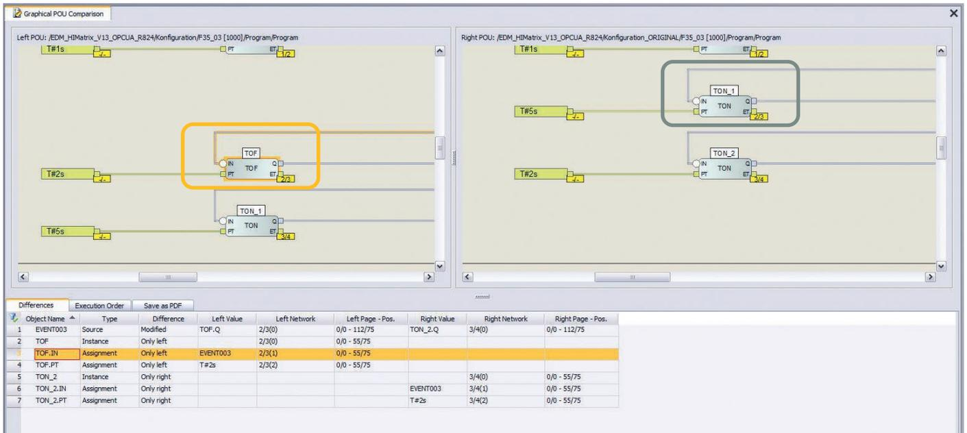
By selecting two different versions of a logic, the differences are highlighted graphically in side-by-side windows and supplemented by details in tabular form.
